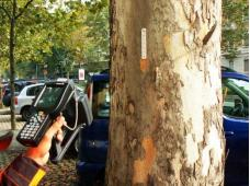
Global Tag RFID and NFC PATCHY is a flexible, strong, waterproof IP68 tag family, designed to be applied directly into the wood for tree tracking, as same as for maintenance purpose in the production plants. It is available in UHF frequency with different IC chip. The silicone surface can be printed with logos and serial numbers.
