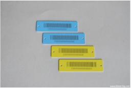
Global Tag RFID UHF **TALLY** is a PVC UHF tag with size 90x25mm. The lateral holes allow an easy and fast application. It has been designed for the tracking of plastic bins for their collection, in order to implement the RFID technology in the sector of the waste management. It can be printed with serial numbers, barcode, QR code, logo, etc...
