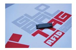
Global Tag **ON-METAL HARDY\_HT6019** is an on-metal UHF tag for high temperature environments which offers high performances. It is the best solution if you need to mount a transponder on a metal surface in industrial environment, where the requirement is to resist to high temperatures (up to 230°C). It has two holes for the mounting.
