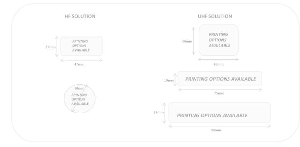
Mounting System: Special Strong Adhesive Weight: 0,5gr. Material: Destructible material Color: White Class Protection: ND Storage Temperature: -25°C to +65°C / -13°F to 149°F Operating Temperature: -20°C to +50°C / -4°F to 122°F Delivery format: in reel Expected lifetime: Some years in normal operating conditions
