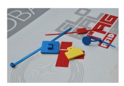
Global Tag **REUSABLE CABLE TIE** is a series of cable tie tags in which the RFID tag and the tail are provided separately; in this way the RFID Tag can be reused and the disposable tie can be wasted. It is available in HF 13.56Mhz, both ISO 14443 (NFC) and ISO 15693 and in UHF 860-960Mhz.
