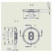
RFID UHF 18mm PPS Button with two holes is a button tag, easy to be mounted with traditional button-hanging machines, which can meet the most complex needs of the laundry tracking projects.
