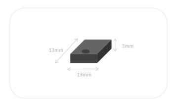
Mounting System: for in-metal solution need to make hole 18x18mm with 4mm depth.
