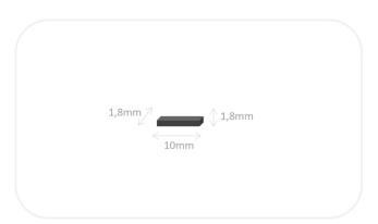
Mounting System: for in-metal solution need to make hole 14x8mm with 4mm depth.
