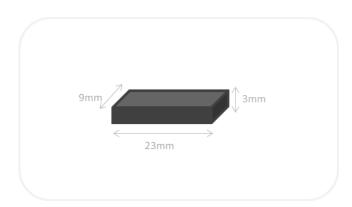
**Mounting System:** for in-metal solution need to make hole 28x13mm with 4mm depth.
