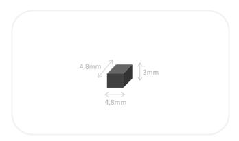
Mounting System: for in-metal solution, it is necessary to make a 6,8mm diameter / 4mm depth mill in the metal object.
