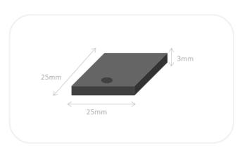
**Mounting System:** for in-metal solution need to make hole 35x35mm with 4mm depth.
