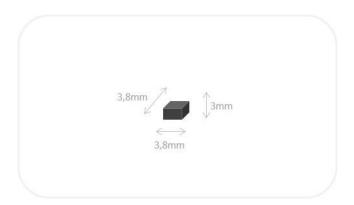
Mounting System: for in-metal solution need to make hole 6mm diameter with 4mm depth.
