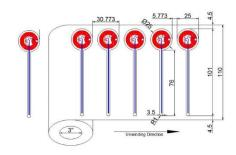
Global Tag **NFC TAMPER EVIDENT LABEL** is a solution which allows to identify an object and get the proof of tampering attempts. Available in NFC, it can be glued on different surface as cartoon, plastic or glass surface.
