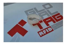
Global Tag **TE-WRISTBY (Tamper-Evident)** is a NFC (HF ISO14443) antitamper wristband, which shows in its memory the tampering attempts.
