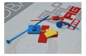
Global Tag **RFID REUSABLE CABLE TIE** is a series of cable tie tags in which the RFID tag and the tail are provided separately; in this way the RFID Tag can be reused and the disposable tie can be wasted. It is available in HF 13.56Mhz, both ISO 14443 (NFC) and ISO 15693 and in UHF 860-960Mhz.
