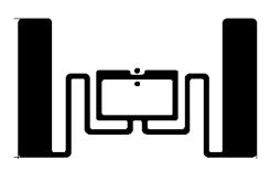
Global Tag **UHF 5030** is a RFID UHF antenna design which has been designed to offer high performance, despite a reasonable dimension. Size of this antenna is 50x30mm.
